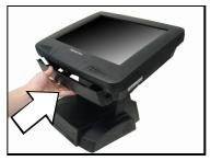
6. Install back the cover for the ports and screw to secure.
