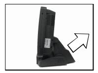
3. Tilt terminal, and pull the back cover upwards to open.
