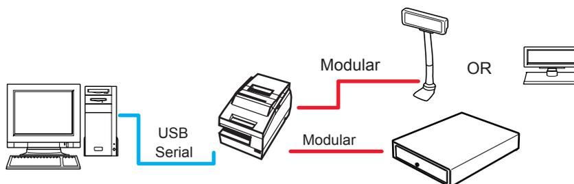
The Y-connection is a connection method to connect the computer and the Customer Display via the TM printer.
