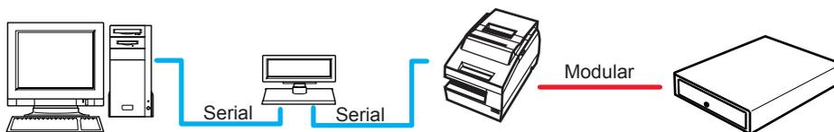
The pass-through connection is a connection method to connect the computer and the TM printer via the Customer Display.
