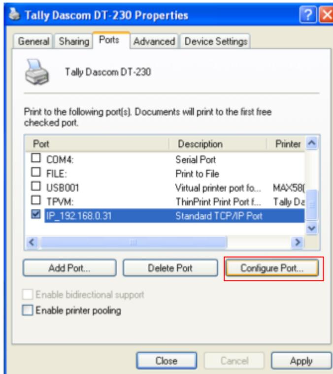
12) Enter the same number as the local port number set during the installation of the interface card in the “Port Number” field in the Raw Settings, and then click [OK] when you finish entering the required values. [Note]Do not change any other items except the RAW Settings.
