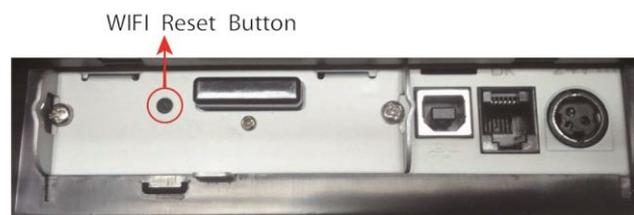
**NOTE: Hold Wi-Fi reset button, at same time power on the printer, Wi-Fi**
