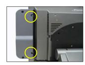
4. Secure the reader with screws (circ)
