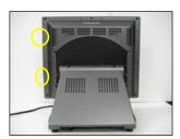
1. Remove screws (circles) to access ports for the reader(s)
