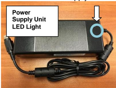
3. Make sure that the power cord is plugged in to the power supply block completely.
